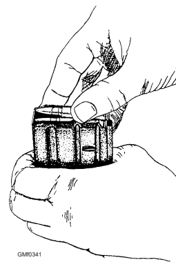
Figure 3-41.—Loading cartridges into the magazine.
